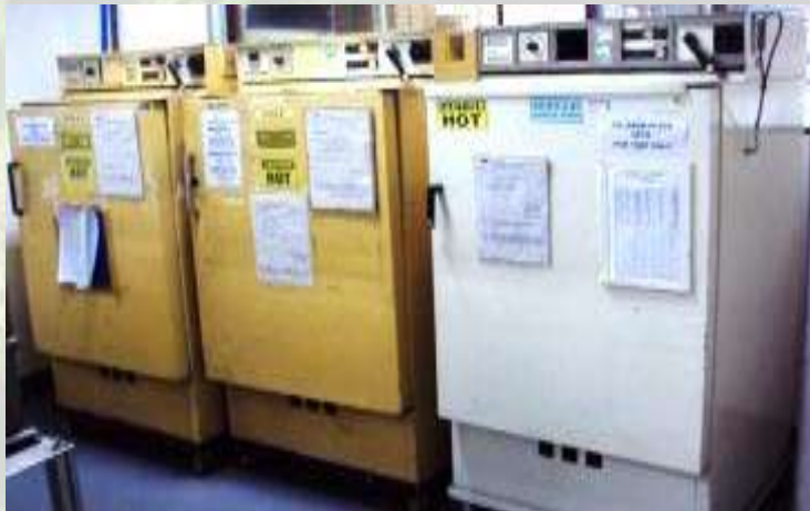
Post curing/ oven drying
